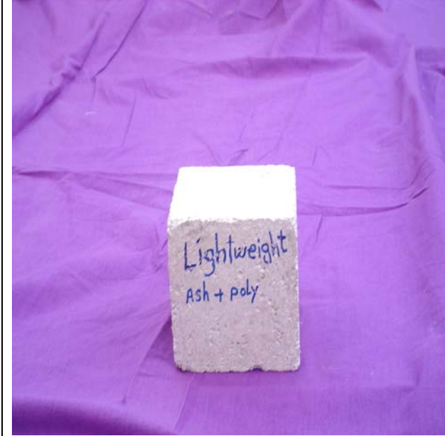
Ultra light weight Ash- polystyrene mix
