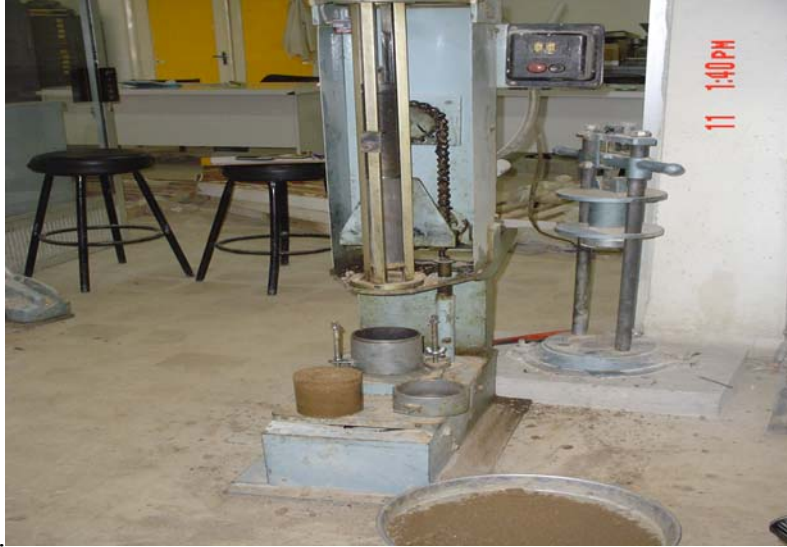
Figure (3) Mechanical compaction machine
